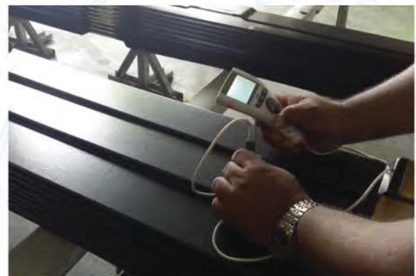
Epoxy Thickness Test
